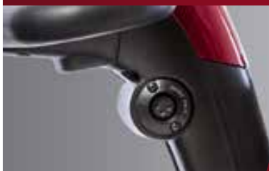
Charger port located conveniently in tiller.
