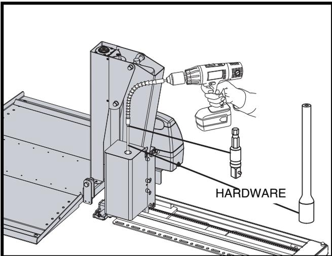
Figure 12. Front-To-Back Movement
