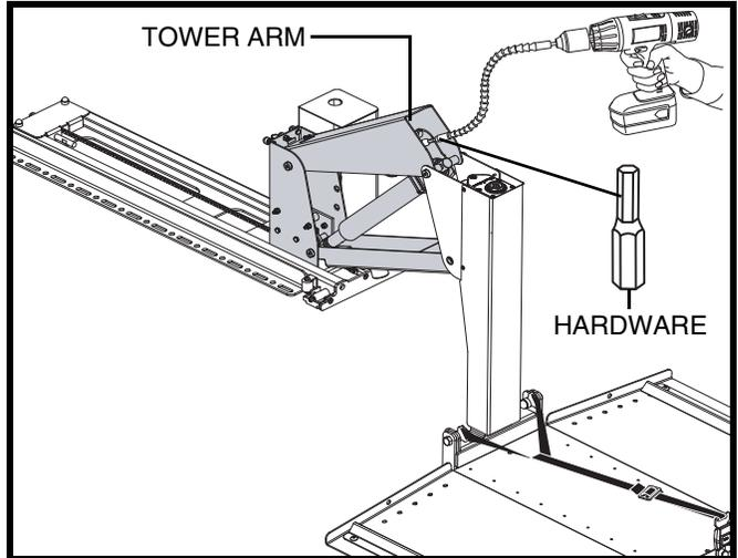
Figure 11. Raise Or Lower The Tower Arm
