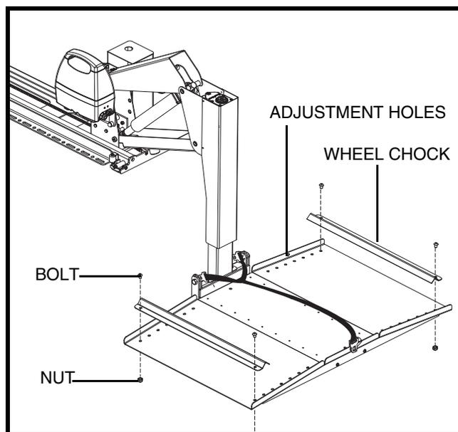
Figure 7. Wheel Chock Installation
