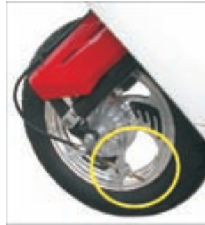
Brake Adjustment Nut Clockwise to Tighten
