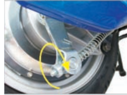
Brake Adjustment Nut Clockwise to Tighten
